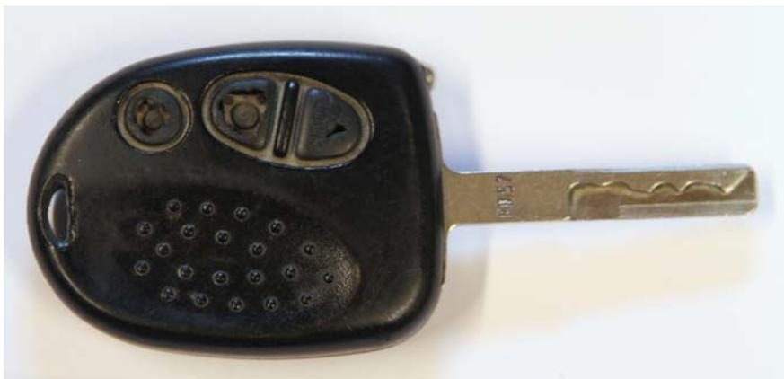
With all of the parts in hand, I got the key from Tom and set off to repair it. As you can see from the before photo above, all three buttons on the key were gone, exposing the switches underneath.
